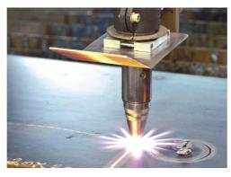
Optionally Oxyfuel cutting is also possible for heavier material.
