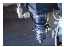
The optional high frequency punch marker permits accurate marking of points and lines.
