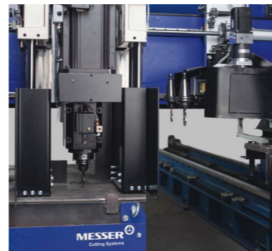
Drilling, boring, countersinking and thread tapping as additional processing possibilities
