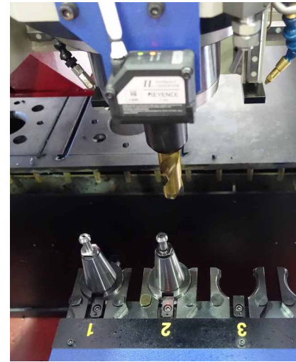
Spindle suitable for outer / inner cutting, equipped with Anti-crash, anti-malfunction laser sensor, Independent oil cooler for BT40 spindle. High machinable harmless mist oil.
