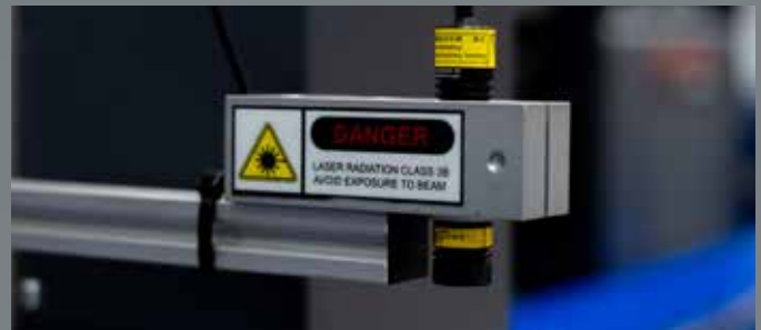
Laser pointer allows the operator to quickly capture the location or angle of the plate.
