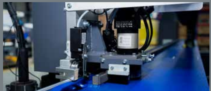
AC servo motors and quality pinions for precise machine movements and uninterrupted operation.
