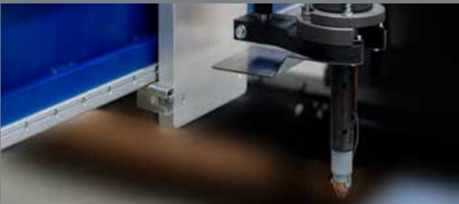
Collision recognition with magnetic torch holder for plasma reduces risk of torch damage
