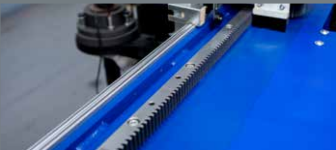
Roller guides provides smooth & precise motion
