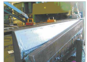
Portacut with 1 torch (standard) cutting a 300mm slab
