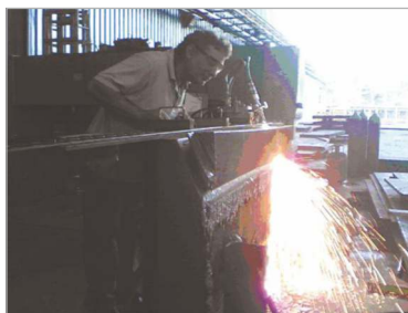
Portacut with 1 torch (standard) cutting a 300mm slab
